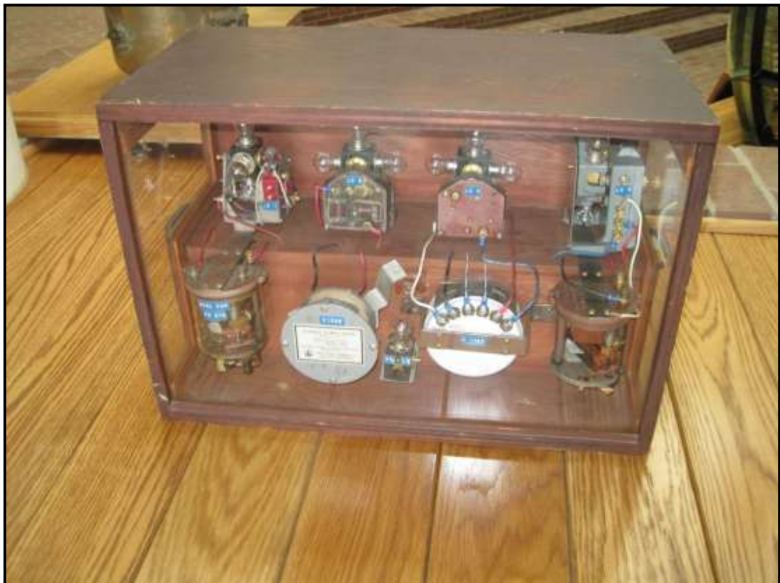
Fig.77 A selection of early lamp changers and flashers displayed in the USCG Aids to Navigation Training School museum.
