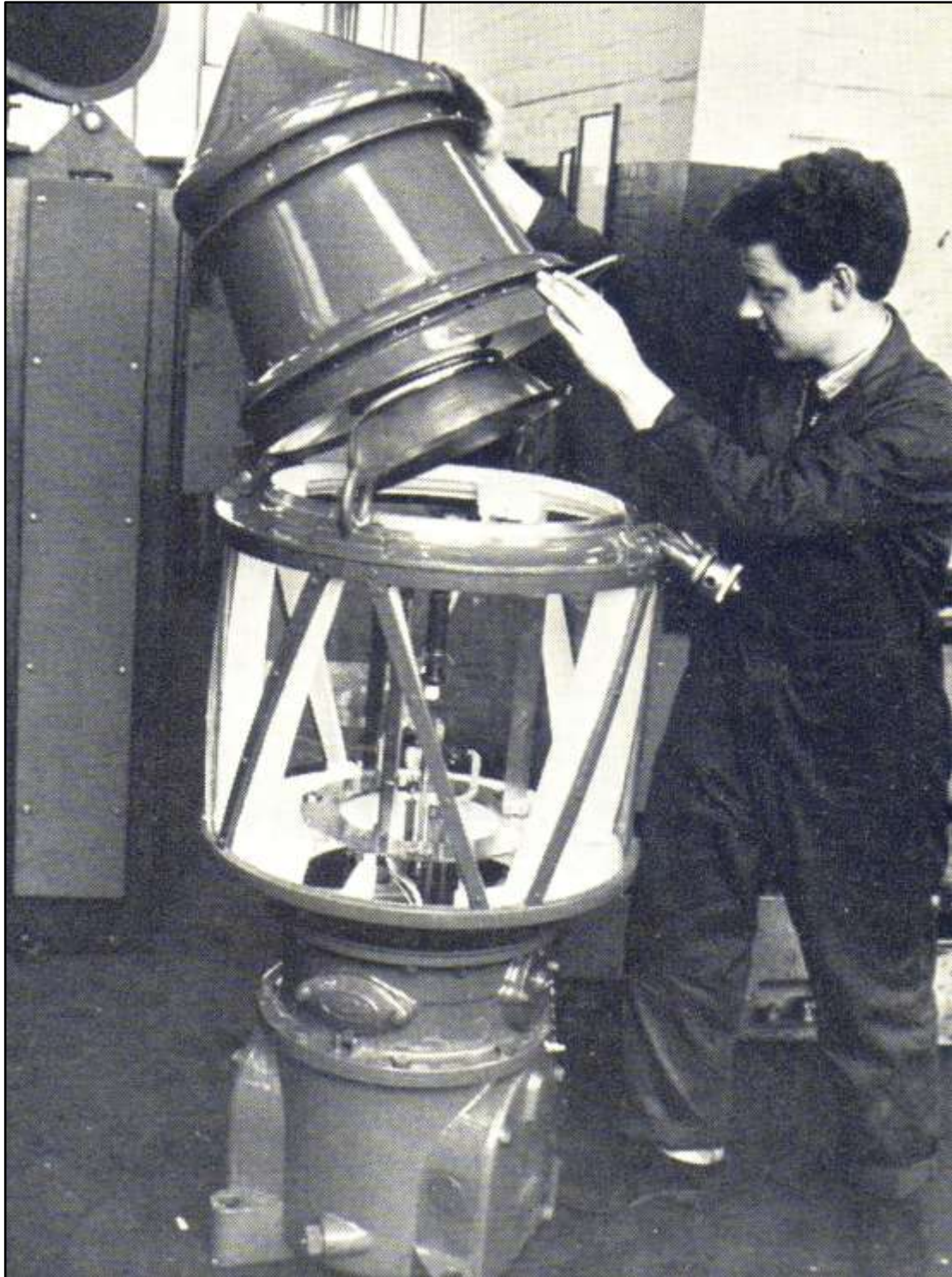
Fig.64 375 mm Dalen lantern Lens not yet fitted
